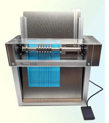
The device is designed as a single sheet cutter. The sample sheet is placed on the metal plate and aligned vertically by means of the knives. When the foot switch is actuated, the sample sheet is grasped, drawn in and the strips are cut. The circular knives and the paper feeder are equipped with a touch protection made of transparent plastic.
