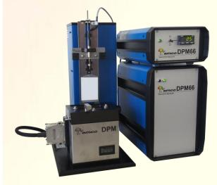
The simultaneous measurement of wet expansion and ultrasonic transmission offers a complex assessment of the paper that is only possible with the *emco* **DPM**.
